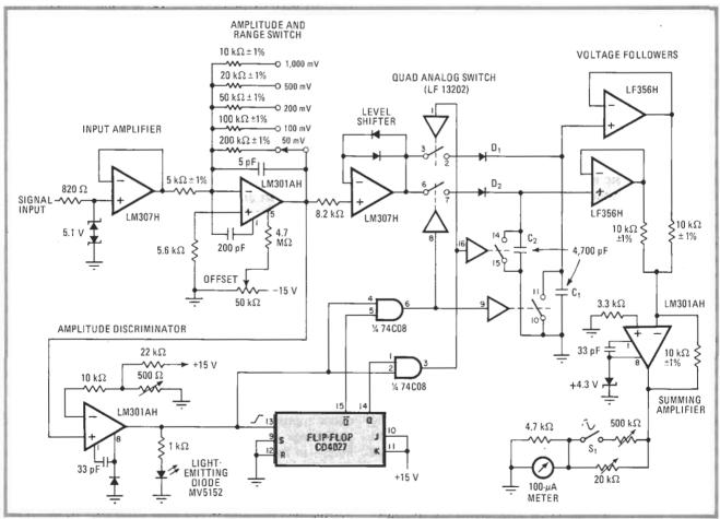
**1. Quick update.** This meter requires only one negative pulse or half cycle of sine-, square-, or triangular-wave input to determine peak current or voltage amplitude. The applied signal charges capacitors  $C_1$  and  $C_2$  alternately, so that either can update immediately without the need for a separate discharge cycle. The meter's range is 0 to 1 V or 0 to 100  $\mu$ A. The output meter reflects instantaneous changes.
